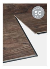
Both Malmo™ Rigid flooring collections utilise the advanced Välinge 5G installation system, making it fast and simple to fit. Even if you're working in tricky or restricted spaces, you can easily achieve a perfect finish as the push down end joints need less positioning space, so there's no need to remove doors whilst fitting. 5G also provides stronger and more stable end joints compared to many other fitting systems.
